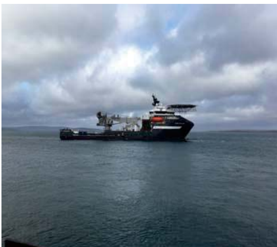
Fig. 2 Larger DP vessel being used for a tidal turbine installation.
